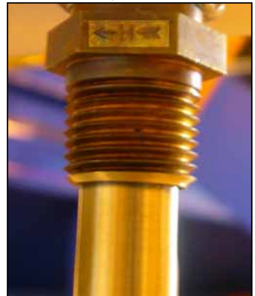
Figure 17: Direction to Turn Screw to Increase Temperature
